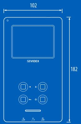
The 6300 series surface mount videophone with a 3.5" Hi-Res full colour active matrix LCD screen is designed primarily for low and high-rise private developments and individual houses where an attractive and low cost functional videophone is desirable.
